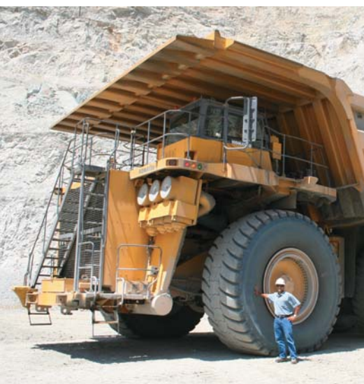
A haul truck that is three stories high and can carry more than 300 tons.
