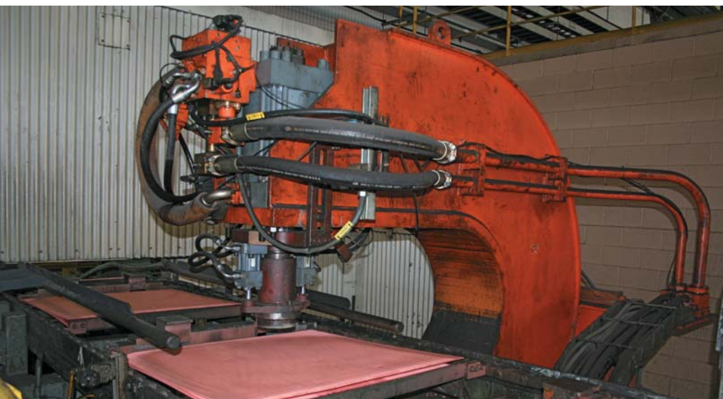
Kennecott punches 1-inch samples out of every other copper cathode as part of its Quality Assurance Program.
